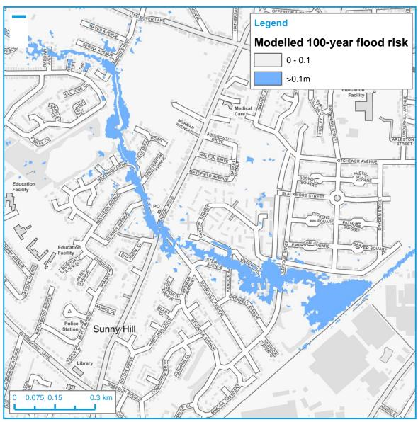
The modelling has shown 235 residential properties at very significant risk of flooding (assuming a property threshold of 0.05m), this falls to 47 if the property threshold is increased to 0.1m. A visual assessment of property thresholds was undertaken using Google Street view mapping and this was verified by Derby City Council staff. It was concluded that in the absence of detailed threshold survey, a 0.05m threshold was appropriate for analysis in this OBC.
